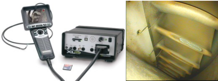
Fig. 13. An industrial videoscope and an image of gas turbine blades condition (Reports, 2000-2010)
