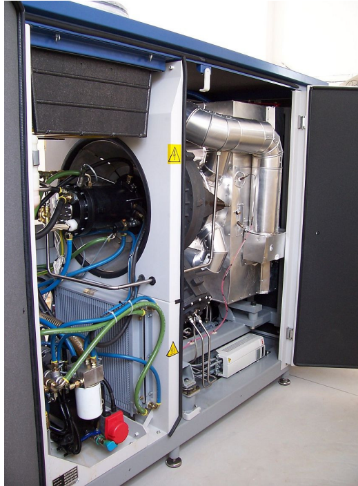
Fig. 2. The T100 power module installed at the laboratory of the University of Genoa (power electronics and control system are not shown).
