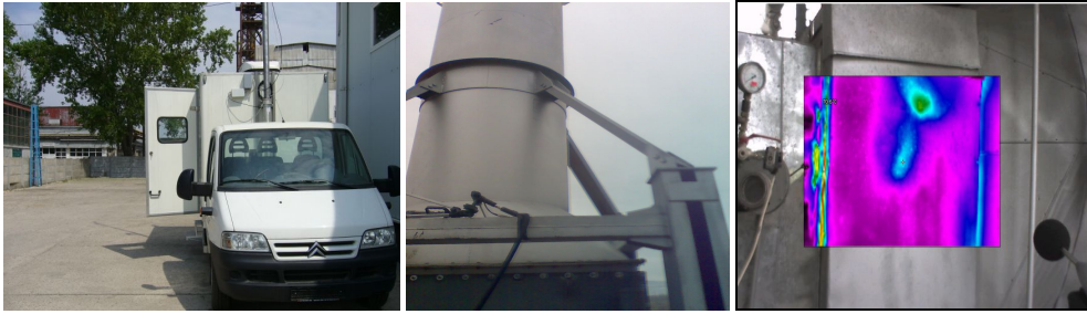
Fig. 13. Mobile laboratory at INCDT COMOTI (left), emissions measurements at the stack (centre) and sighting area of Fluke camera (Ti45FT type) with sound level meter (right)
