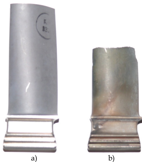
Fig. 15. Gas turbine blades : a) – the new one, b) – the in-service damaged one, magn. \times 0.75
