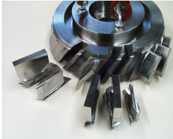
Fig. 26. Pre-machined BLISK demonstrator, after extraction of blade-blocks.
